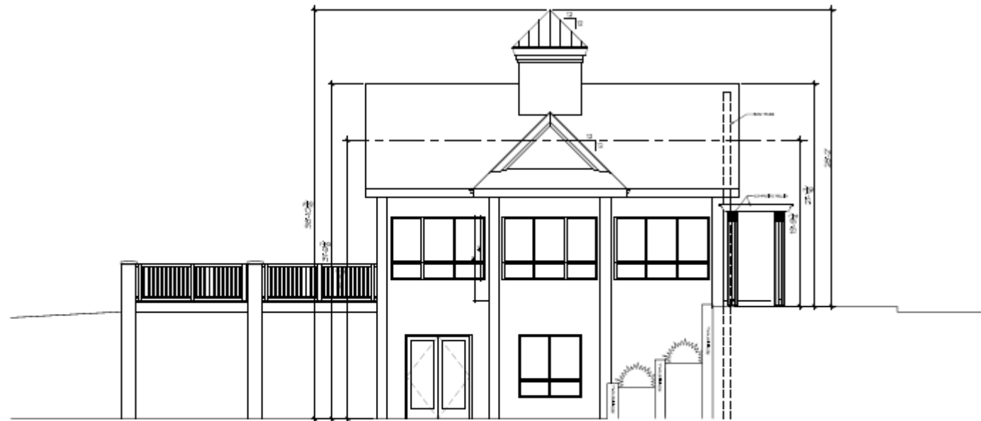
North Elevation - Pavilion 3/16"=1'-0"
