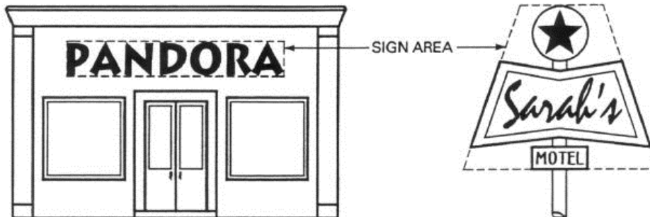
Figure VIII-10 Examples of Measurement of Sign Area
