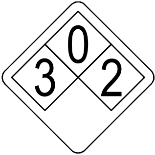
ALERTING SIGN (FOR CELL SITE BATTERIES)
