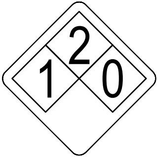
ALERTING SIGN (FOR DIESEL FUEL)
